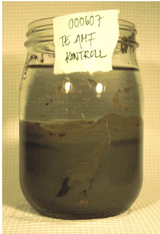
Fig. 1. Experimental jar. Anoxic base sediment covered by a top layer of oxic sediment (light layer) enriched to an OC content of 3% with either lignin or Tetraselmis spp. (a green flagellate). The light colored sediment in the dark anoxic sediment layer shows the burrow linings of A. filiformis .
